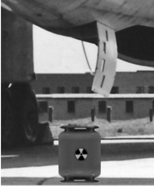
RADHAZ container on ground and shown installed in a Valiant airframe. ©Pete Sharp
