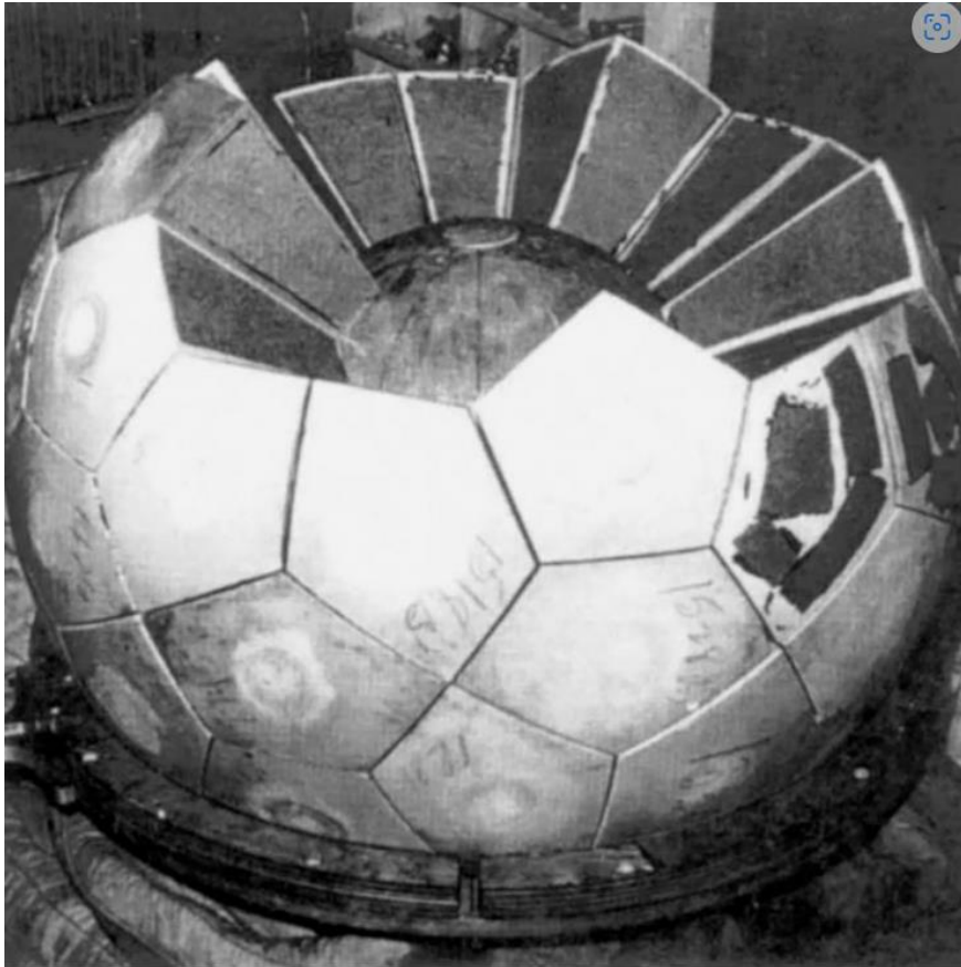
Physics package showing HE lenses and pusher sphere © Pete Sharp
