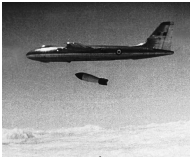
Second prototype Valiant WB 215 releasing an inert ballistic test weapon over Orford Ness © Crown copyright
