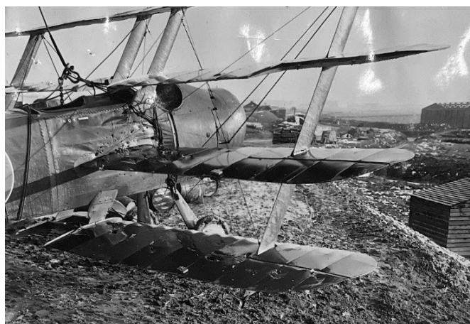
Armstrong Whitworth F.K. 10 battle damage test on Orford Ness (Crown Copyright)
