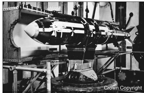
WE177 mounted on electro/mechanical vibrator within local thermal chamber
